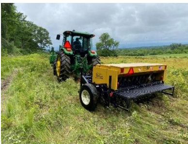
Photo of the tractor and no-till drill planting in Terry Berry grassland (photo credit USFS Greg Flood)
